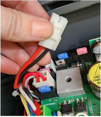
Once the power to the barrier has been completely disconnected, plug the socket back into its position and plug back the mains power to the barrier.
