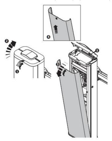
• Tilt the barrier door forward and left out of position (sequence 3 and 4).
