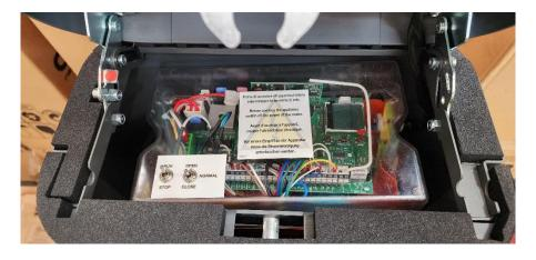
• Remove the battery backup pin socket (white connector with red/black wire) as indicated in image.
